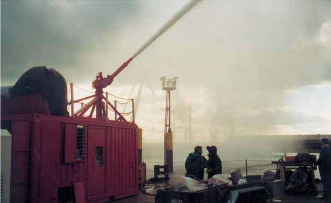
The unit during a 24-hour test program (pump 1200 m<sup>3</sup>/h - 16 bar)
