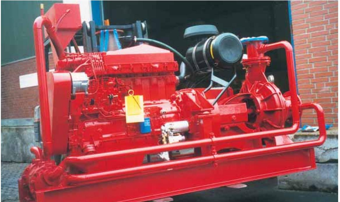
Stationary marine design with Scan engine, pump made of NiAl-bronze 360 m<sup>3</sup>/h – 140 m
