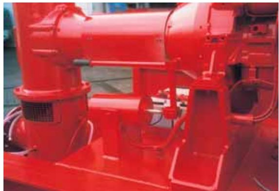
We deliver, if required, with clutch for automatic remote operation with emergency manual operation
