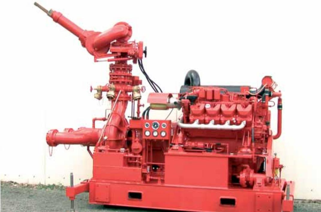
Pump capacity 12000 l/min at 13 bar
