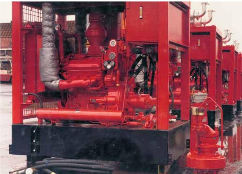
Hydraulically driven power package for submersible pump
