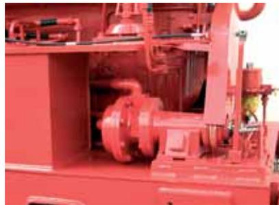
Evacuating system with high capacity (evacuating time can be less than 1 minute) pump made of bronze, operating by hand lever to disk clutch
