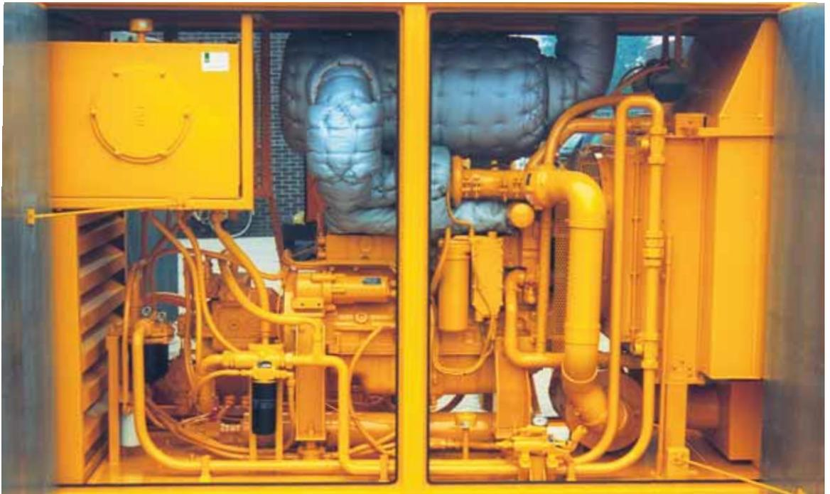
Diesel driven hydraulic power package
