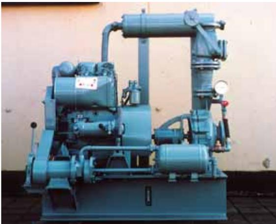
Diesel-driven centrifugal pumps with 3-cylinder Deutz-engine with separate evacuating device with clutch for manual operation
