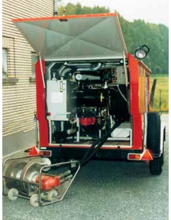
Hydraulically driven mobile power package with floating submersible pump
