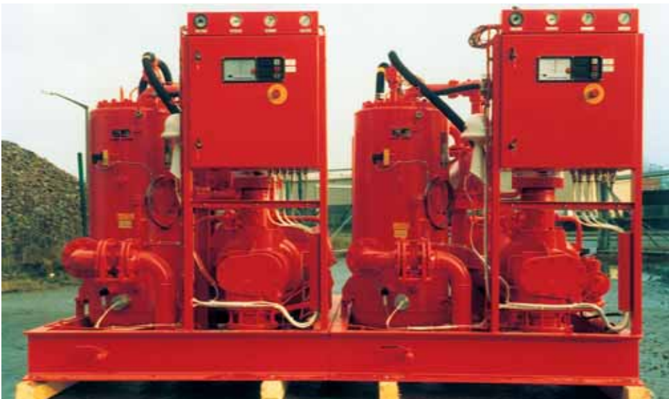
Double working air screw compressor unit
