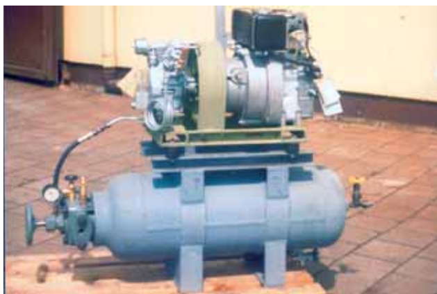
Emergency starting compressor
